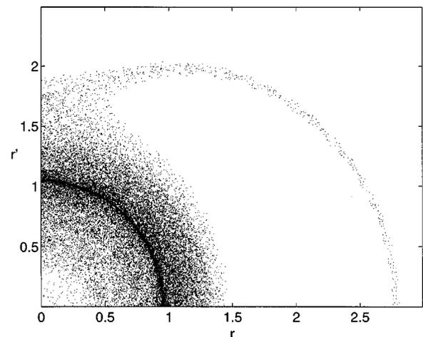
FIG. 5. Stroboscopic plot in the transverse phase space for 125 particles with low angular momenta. The dark elliptical arc corresponds to the initial distribution ( $\eta=0.7$ ,  $\mu=0.8$ ).
