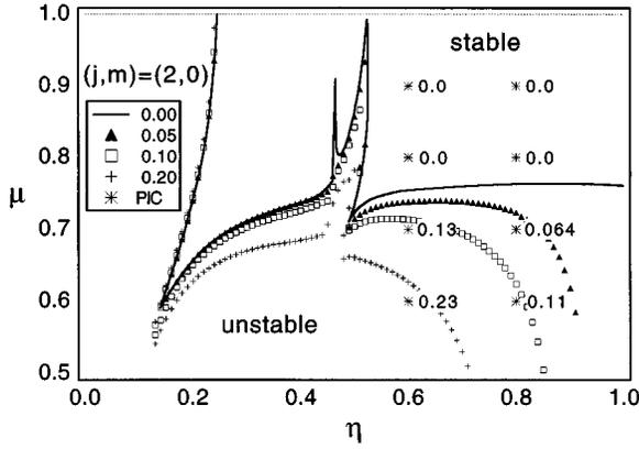
FIG. 1. Stability limits and growth rates for the  $j=2, m=0$  mode in the mismatch ( $\mu$ ) tune depression ( $\eta$ ) space. Contours for growth rates of 0.05, 0.10, and 0.20 are shown, as well as growth rates obtained from particle-in-cell (PIC) simulations.
