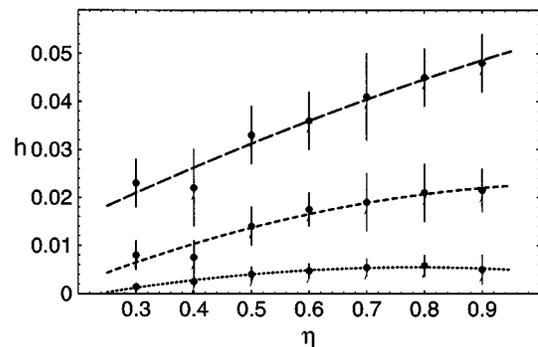
FIG. 9. Halo intensity vs tune depression  $\eta$ : long-dashed line,  $\mu=0.6$ ; short-dashed line,  $\mu=0.7$ ; and dotted line,  $\mu=0.8$ . Points with error bars are from simulations, curves fit the data.
